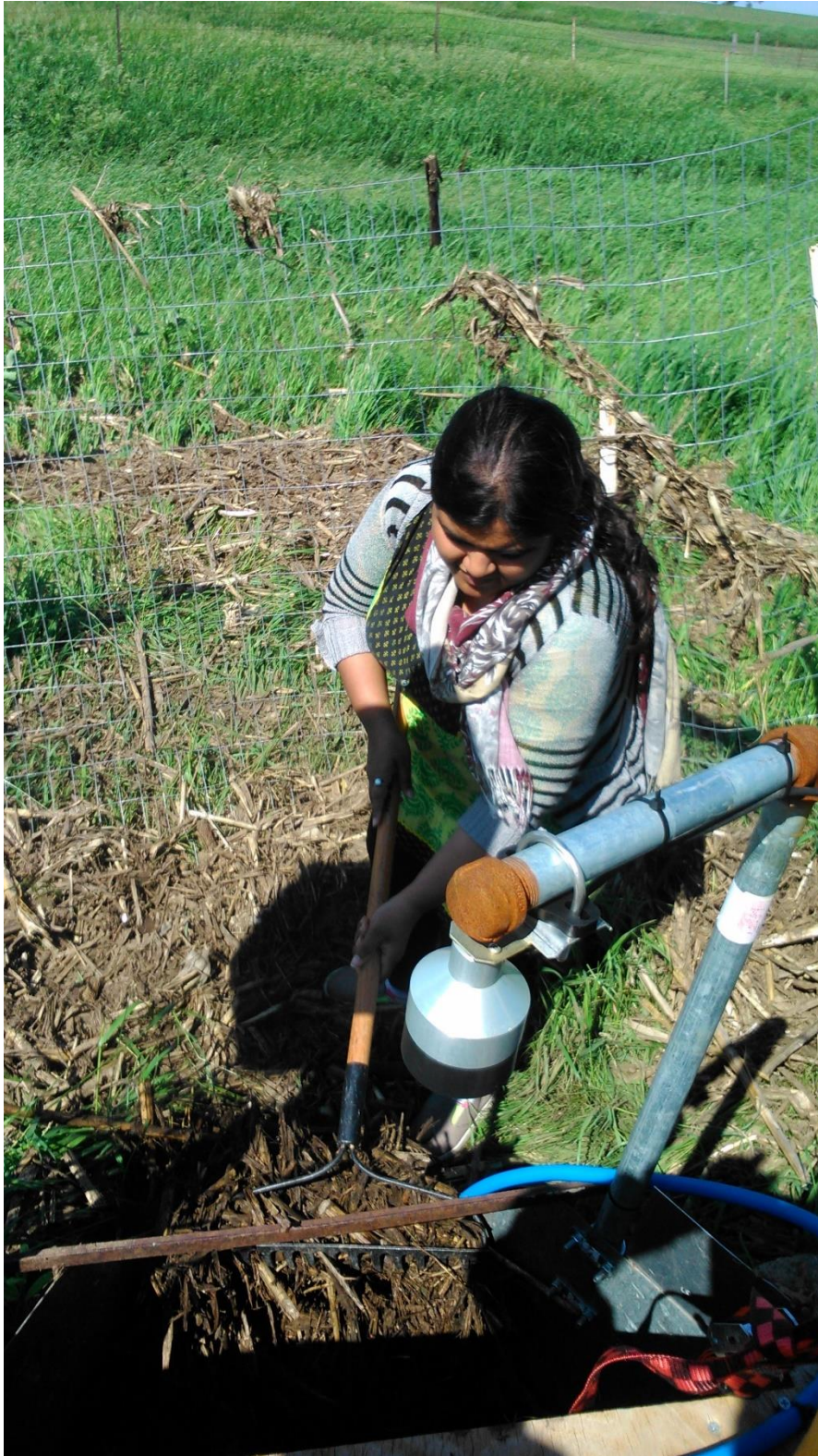
Figure 3.5.3. Cleaning the clogged flume after the storm events
