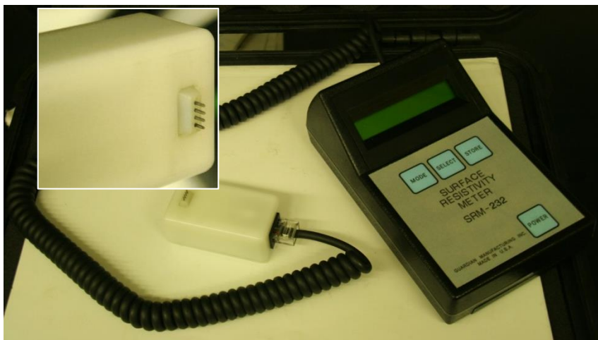
Figure 3.21. Photograph of Guardian SRM - 232 - 100 used to measure sheet resistance with an inset of the probes.
