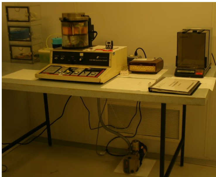
Figure 3.23. Photograph of Plasma Sciences Inc. CrC-150 Sputtering System used to deposit gold.
