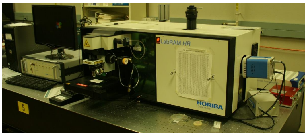
Figure 3.9. Photograph of LabRam HR800 system used for Raman spectroscopy.
