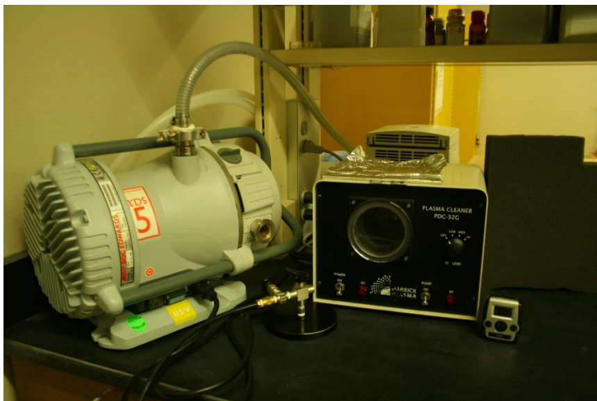
Figure 3.1. Photograph of plasma cleaning set up with a BOC Edwards XDS5 vacuum pump on the right and a PDC-32G plasma cleaner on the left.
