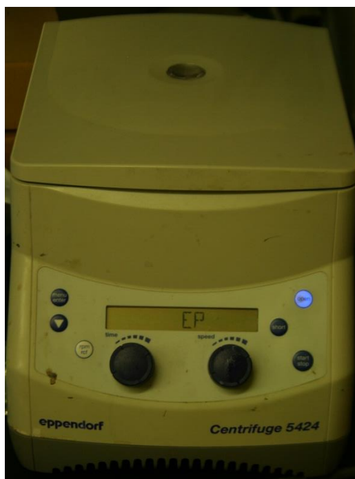
Figure 3.18. Photograph of Eppendorf Centrifuge 5424 used to clean silver nanowires.
