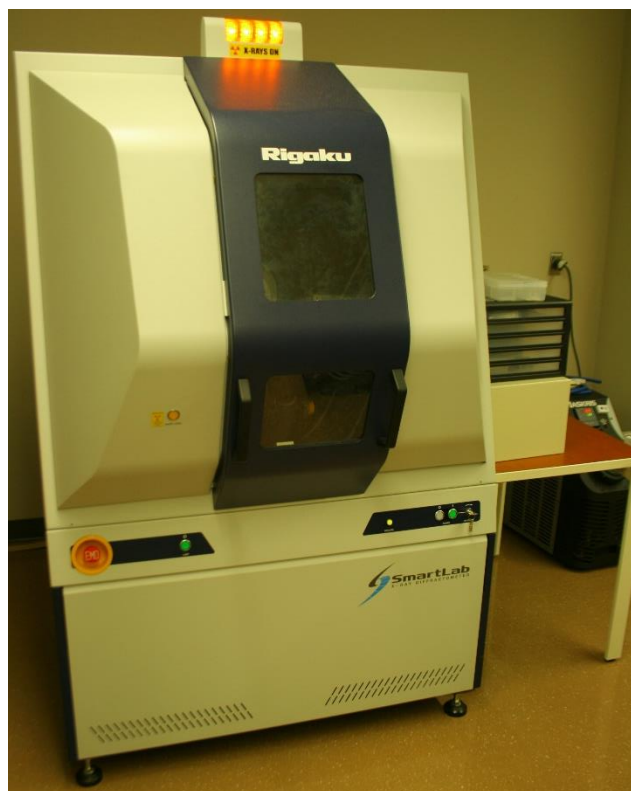
Figure 3.13. Photograph of Rigaku Smartlab system used to obtain X-Ray Diffraction (XRD) spectrum.
