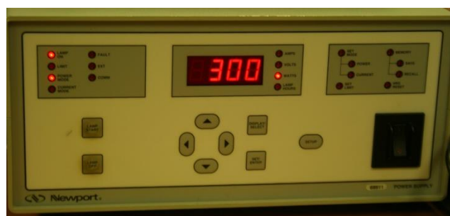
Figure 3.15. Photograph of Newport 69911 power supply used to power the Xenon Arc lamp.
