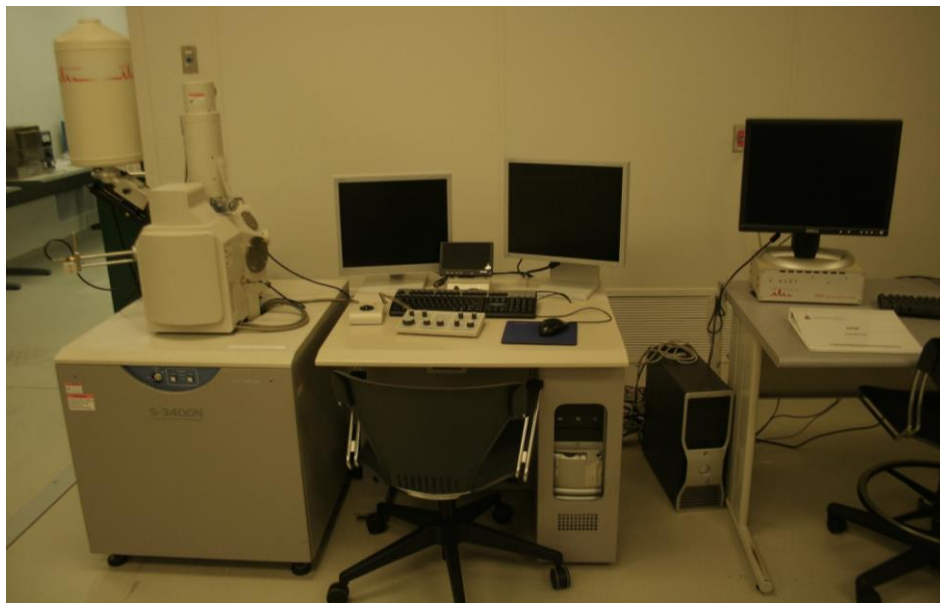
Figure 3.6. Photograph of Hitachi S-3400N system used for SEM imaging and EDX measurements.
