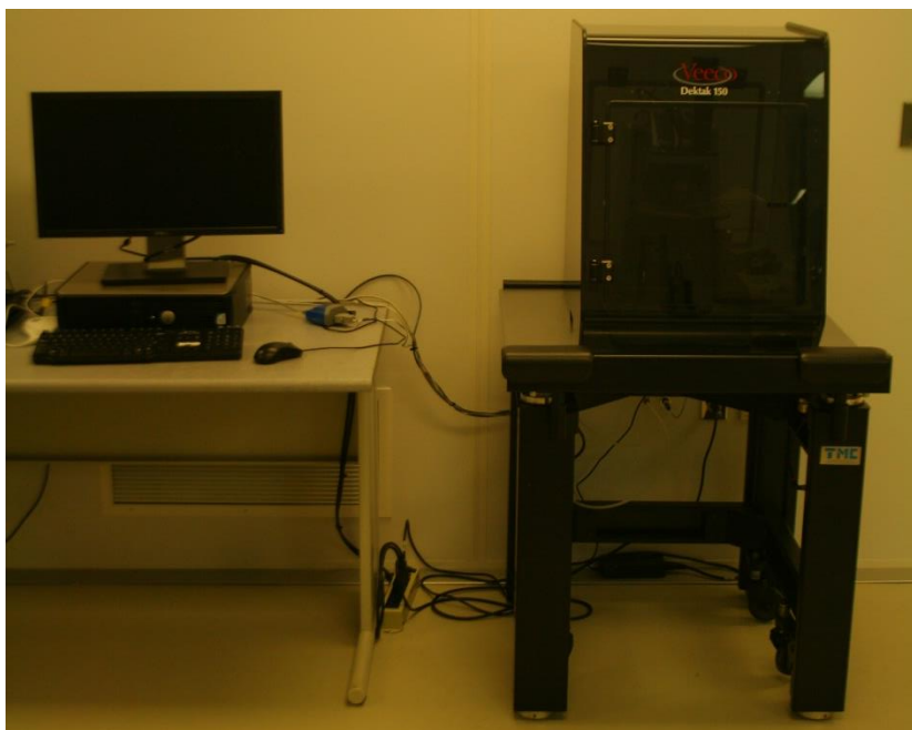
Figure 3.3. Photograph of Veeco Dektak 150 used to measure film thickness.
