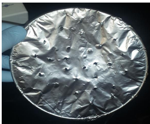
Figure 3.15. CGPE coated PP separators in Petri dishes covered by aluminum foil with holes.
