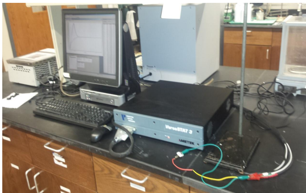
Figure 3.18. System setup used for Electrochemical Impedance Spectroscopy (EIS) and Cyclic Voltammetry (CV).
