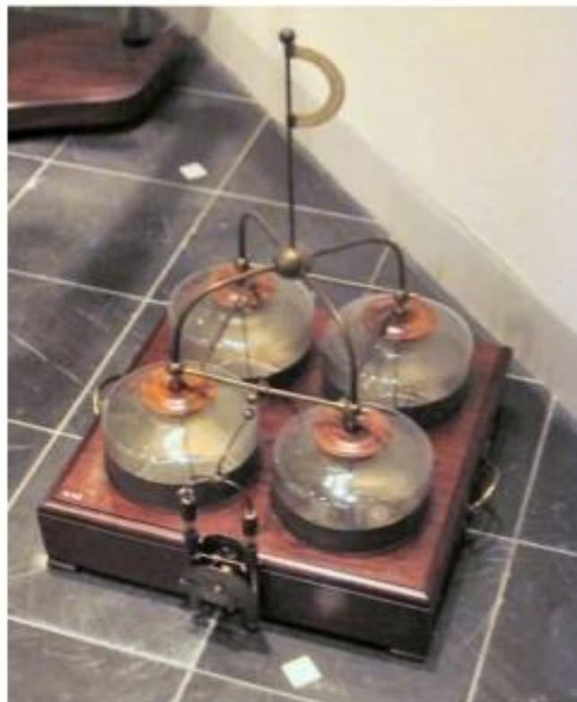
Figure 1.9. Franklin battery made of a series of connected capacitors [20].
