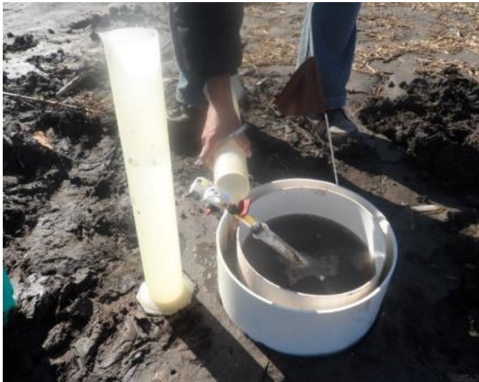
Figure 4.1 Infiltration measurement at White Lake, SD.
