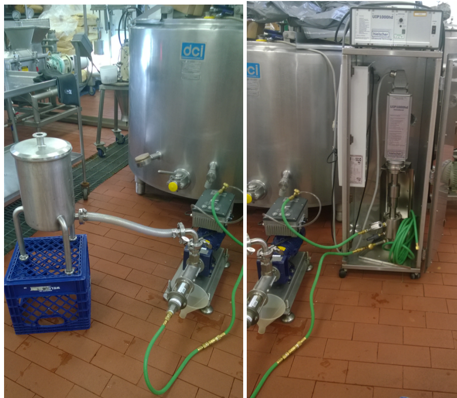
Figure 5. Ultrasonication treatment setup in R&D section of Davis Dairy Plant with inlet dosing tank, ultrasonication unit with an outlet line.
