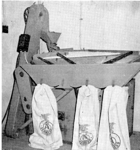
Figure 2. A gravity table. It separates seeds by weight. Light seeds are discharged at the left front and heavy seeds at the right front.
