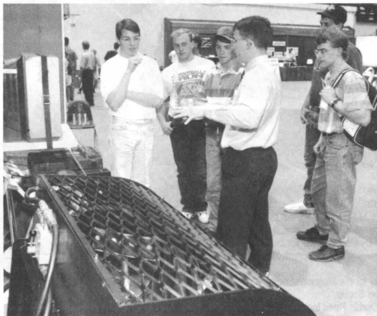
Darren Fehr explains the SkidMix, a multi-purpose mixer used as a skid steer attachment, to a group of students during Engineering Exploration Days.
