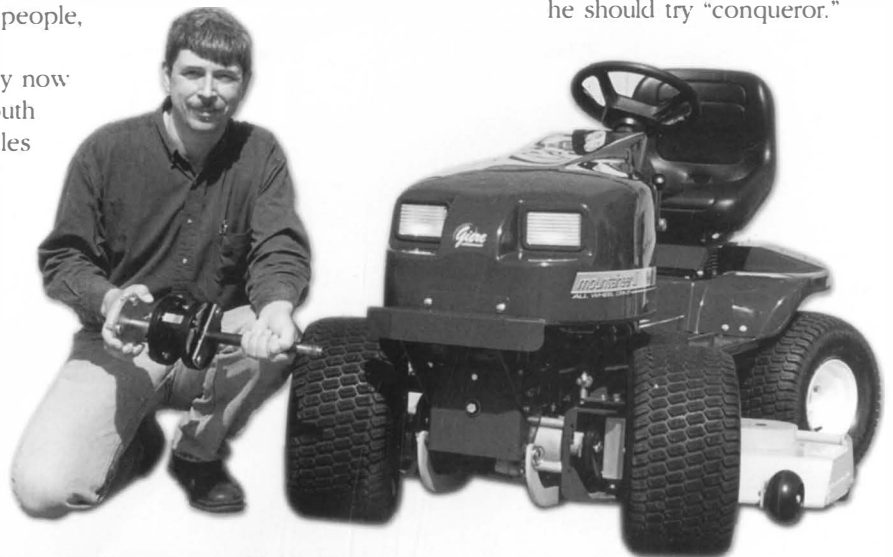
David Giere poses with his Mountaineer lawn tractor while holding the patented flexible coupling that allows the mower to have four-wheel drive, four-wheel steering, and four-wheel braking.
