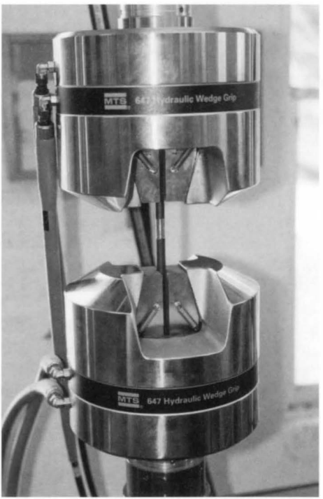
ABOVE: The five primary pieces of the MTS 810 system. Clockwise, from upper left, a personal computer, a load unit assembly, a remote station control panel, a hydraulic power unit, and a digital controller. BELOW: With a vice grip hold, the hydraulic wedge secures a steel rod for strength testing. The machine allows fatigue studies on nearly every type of material. From titanium to advanced ceramics and plastics.
