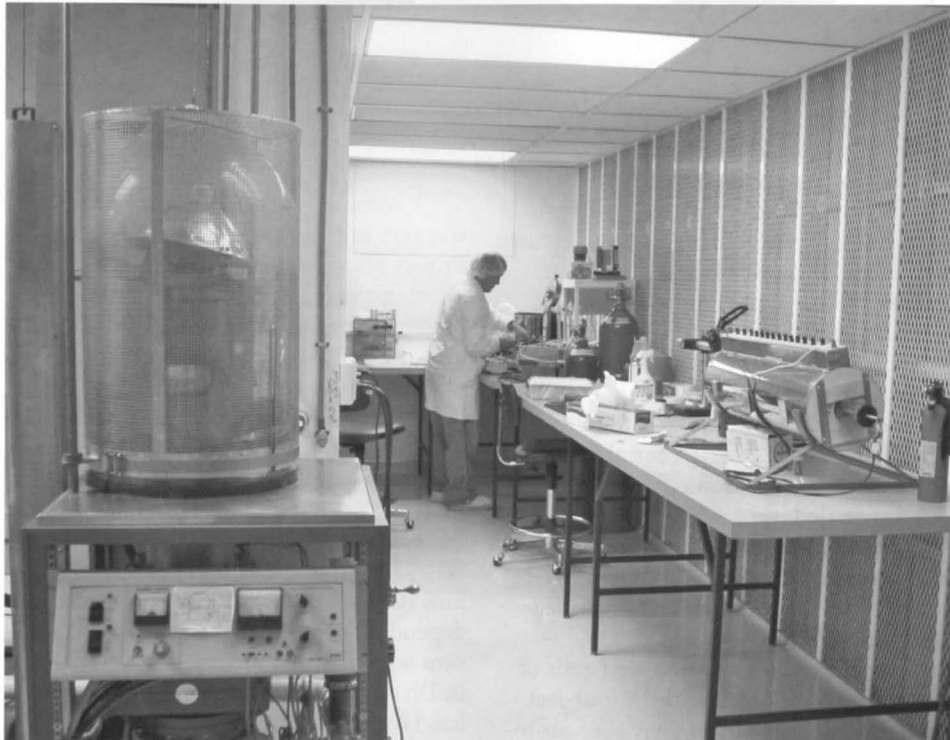
Jeff Moore, cleanroom technician in the Department of Electrical Engineering and Computer Science, works on the RF sputtering system in the Solberg Hall Annex. The RF sputtering system allows well-controlled deposition of thin films of materials. The lab, originated in 1982 and expanded in 1992, will be the site of much of the research work associated with a new doctorate in electrical engineering.
