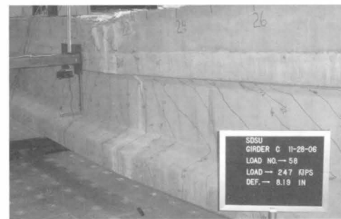
TOP: The girder arrives on a flatbed. BOTTOM: A girder right after failure.
