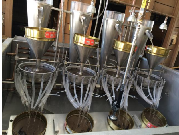
Fig. 2.1. Mechanical elutriator used for extraction of females (cysts) from soil samples collected from the soybean fields.
