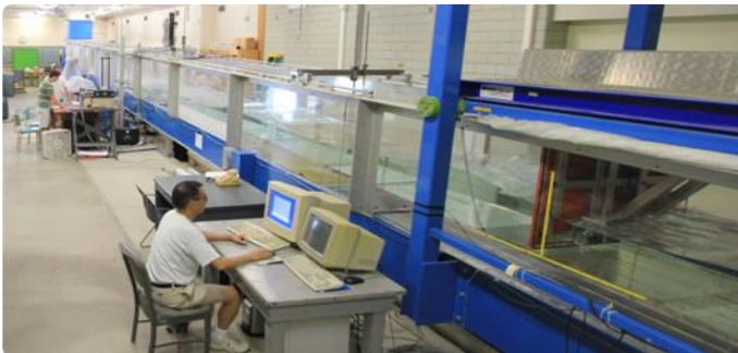
Figure 1. Experimental setup with open-channel flume and wave generator
