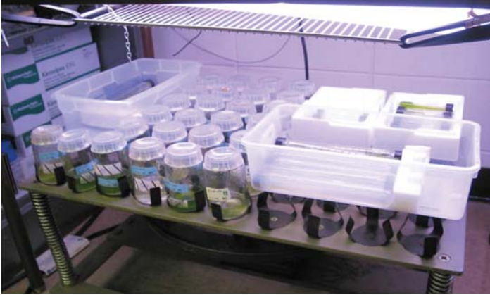
Figure 1. Algae cultures grown on a shaking table under fluorescent light. Cells were kept constantly shaking and on a 16/8 photoperiod. Different volumes of cells including 6 mL cultures and 50 mL cultures were grown.
