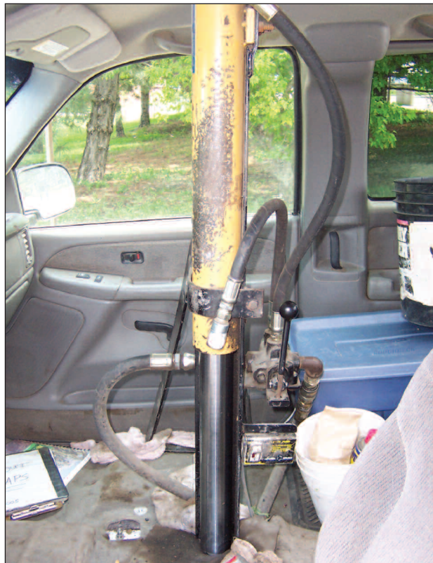
Fig 3. In-cab truck mount hydraulic probe.
