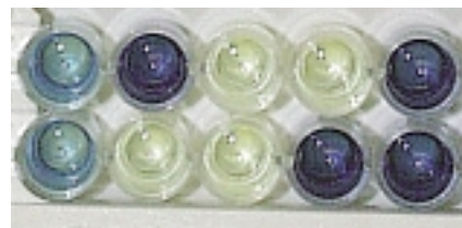
Figure 4: An ELISA test can detect very small quantities of specific contaminants in grain. The development of color (blue in this test) indicate the presence of the toxin. Intensity of the color can indicate the amount of toxin present. Photo: M. A. Draper.
