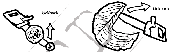
Figure 8. Kickback is a common cause of chainsaw injury to an operator. Hitting an object with the nose of the moving chain will throw hundreds of rapidly moving blades at you. Do not operate your saw beyond your capacity of experience. Ask your chainsaw dealer for the safety rules published by the Chain Saw Manufacturers Association.
