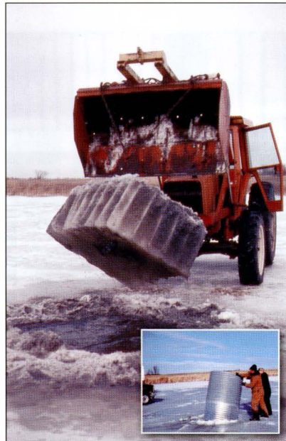
Ice was lifted out using a tractor-loader and chain.
