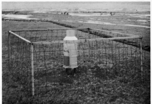
Figure 5. Recording rain gauge, Range and Livestock Experiment Station, Cottonwood, South Dakota.
