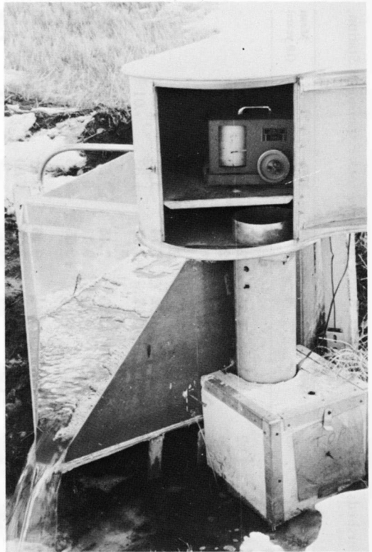
Figure 4. H-type flume with stage recorder measuring snowmelt runoff from one high range condition watershed, Range and Livestock Experiment Station, Cottonwood, South Dakota.
