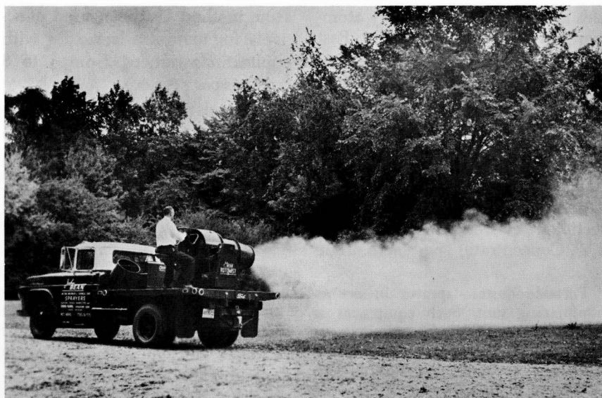
Heavy duty mist-blower in use for larviciding. Such machines employ high-velocity air blasts to disperse insecticide, and can be used for adulticiding as well as larviciding. (Photo courtesy John Bean division, FMC Corp., Lansing, Mich.)
