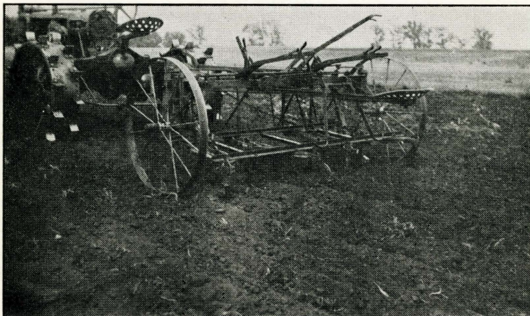
The ordinary two-row cultivator converted into a weed control machine and substituting for the field cultivator on small areas.
