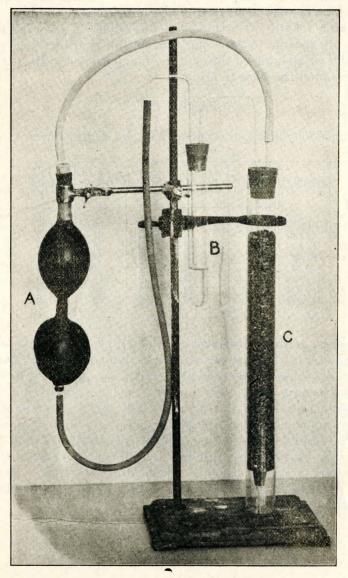
APPARATUS FOR APPLYING VAPORS TO SEED GRAIN A. Hand-blower for producing a current of air. B. Test-tube containing fungicide in liquid form. C. Cylinder containing seed grain.
