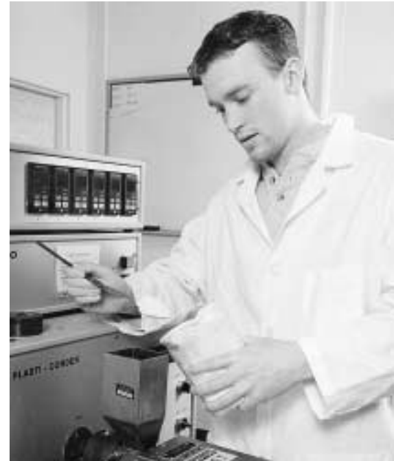
Troy Small, Blaine, Minn., undergraduate research assistant, adds corn flour to an extruder in a project to find an ag product alternative to petroleum.
