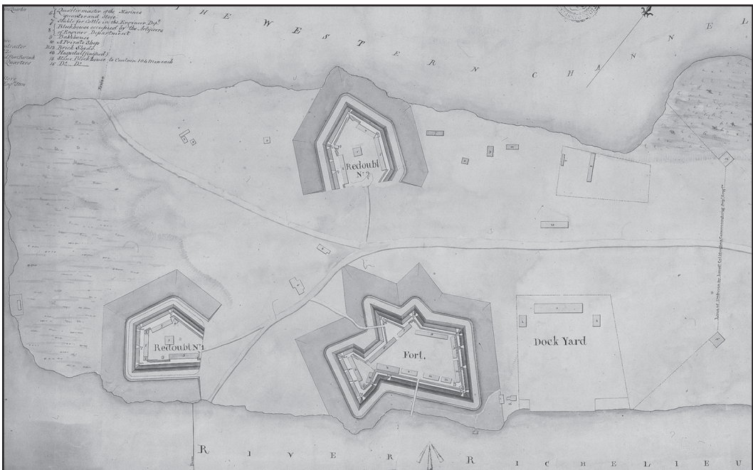
Figure 12. Detail of A Plan of the Works at Isle aux Noix , known as the Hughes Plan (1814), showing restoration work of 1812–1814. The northeast redoubt has been demolished, and back walls from the two remaining redoubts have been replaced by wooden palisades. Water-filled ditches surrounding the redoubts have disappeared.
