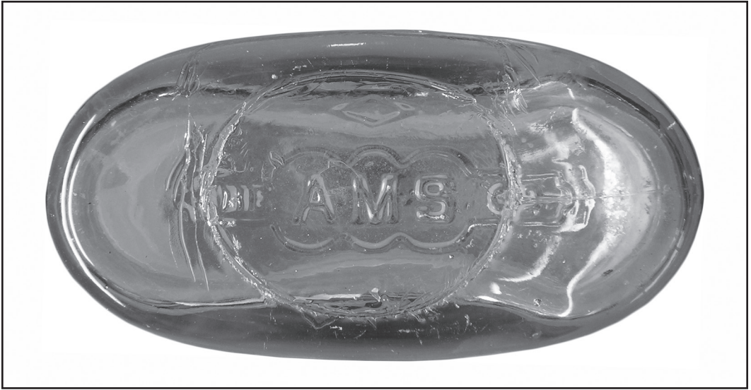
Figure 7. Owens suction scar on a “FULL PINT,” cork-stopped, colorless glass liquor flask. There is a faint Illinois Glass Co. I-Diamond trademark above the bottler’s mark: THE A.M.S. CO. (the American Medical Spirits Co.) which made medicinal whiskey during Prohibition. This information, plus the I-Diamond mark, dates the bottle to between 1919 and 1929. Notice the slightly oval mark, which is from the blank mold. The knife cutting off the glass created the Owens scar, dragging some of it off to the left side of the oval blank mold mark. (Photo by George L. Miller, 2013.)
