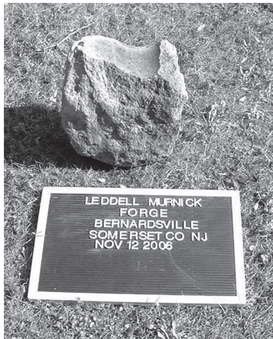
Figure 14. A granite bearing block to support a water-wheel axle or cam shaft.
