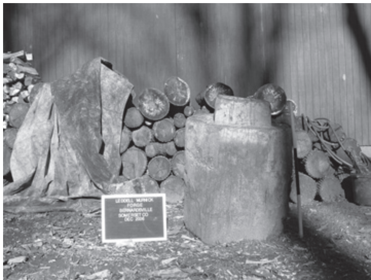
Figure 7. The anvil base showing the large tenon.
