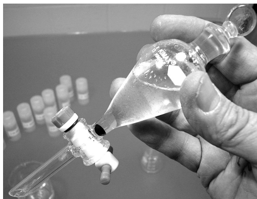
Figure 16. Flotation with heavy liquid showing glass bead descended with garnets collecting at stopcock.
