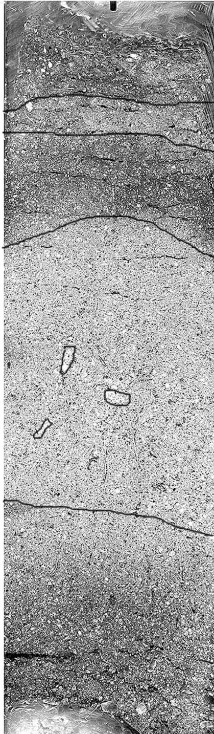
Figure 3. Scanned image of Core 1. Labeled on the left is Layer A, which was recorded as a single layer of soil during excavations. Labeled on the right are descriptions of the five soil strata that were discovered in the lab.
