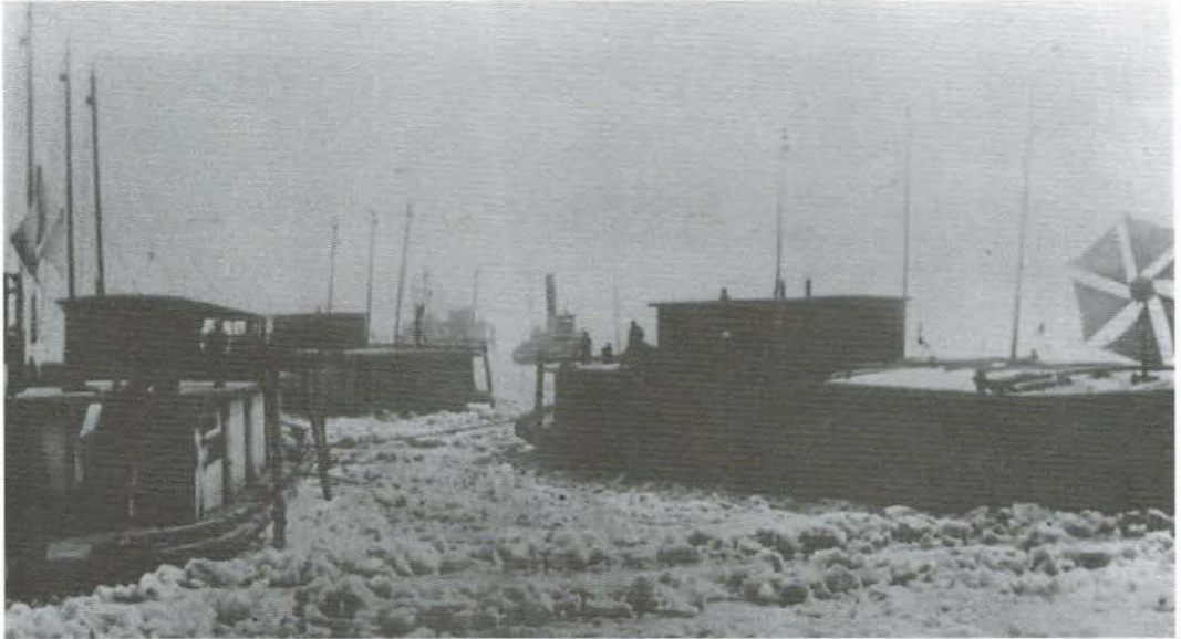
Figure 26. An undated photograph shows a group of ice barges belonging to the Rockland Lake Ice Company. These are shorter and more blunt-bowed than the standard ice barge shown in Figure 24, and have only three derricks. (Courtesy of the South Street Seaport Museum Library.)
