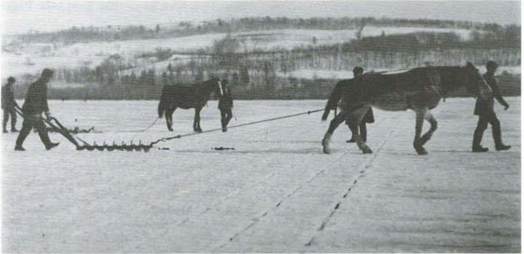
Figure 2. Undated photograph of Hudson River ice crew marking the ice prior to cutting, near Catskill, NY. (Courtesy of the Vedder Memorial Library, Greene County Historical Society.)
