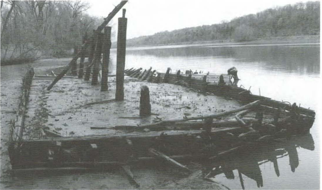
Figure 23. Remains of a wooden barge located near Ice House A (the J. Scott & Company Ice House). A series of upright supports can be seen, attached to the center beam or keelson, which is buried in river silts. The iron bales topping the uprights supported transverse beams, one of which is still present. Deck planking would have been attached to these beams. The view is towards the north.
