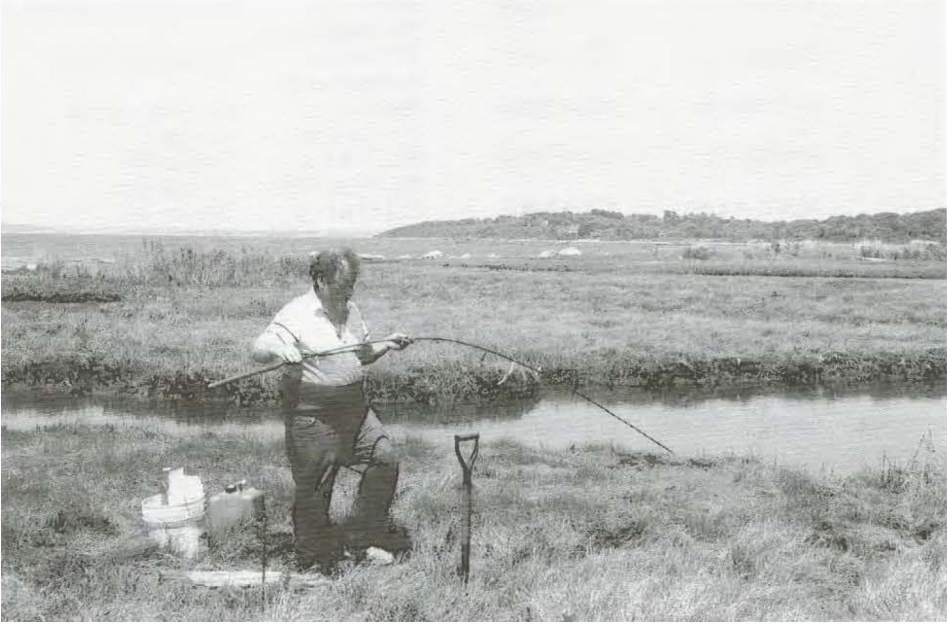
Figure 8. View of Nelson Salt Marsh looking northeast. Pollen samples are being collected using a Davis borer (1990 field season).
