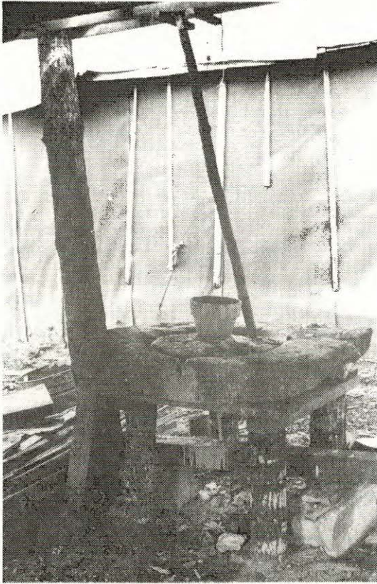
Figure 1. Meaders Pottery glaze mill (potter's quern) once used to mix and refine alkaline glaze, now retired. Upper stone "runner" rests on vertical shaft which can be adjusted to change fineness of grind; photograph shows how upper end of handle is boxed into framing of kiln shelter.
