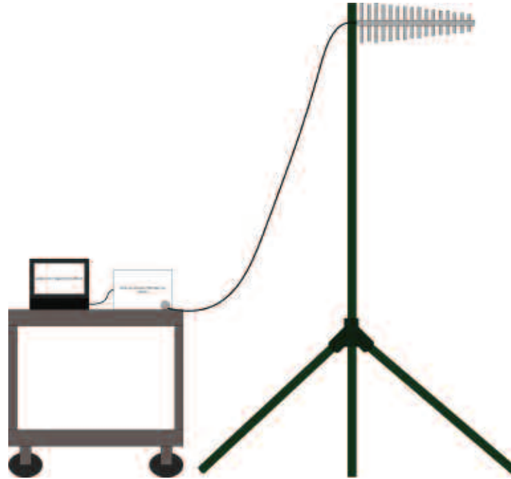
Figure 44: Drawing of the spectrum analyzer power measurement setup
