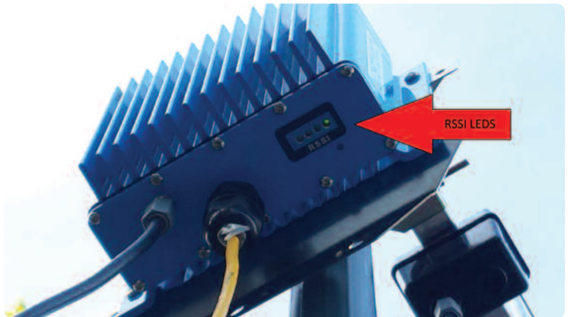
Figure 48: Close up of CPE RSSI LEDs
