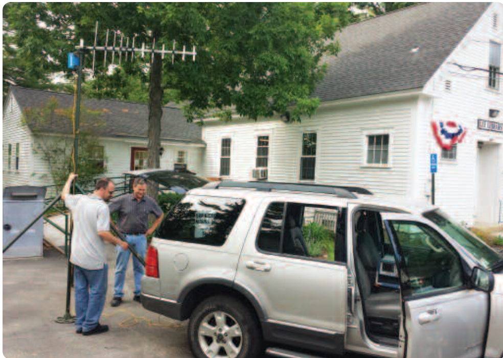
Figure 24: Lee parking lot setup with SUV “ground plane”
