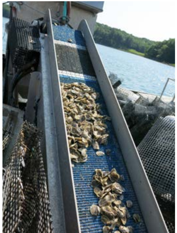
This machine filters the oysters based on their size.
