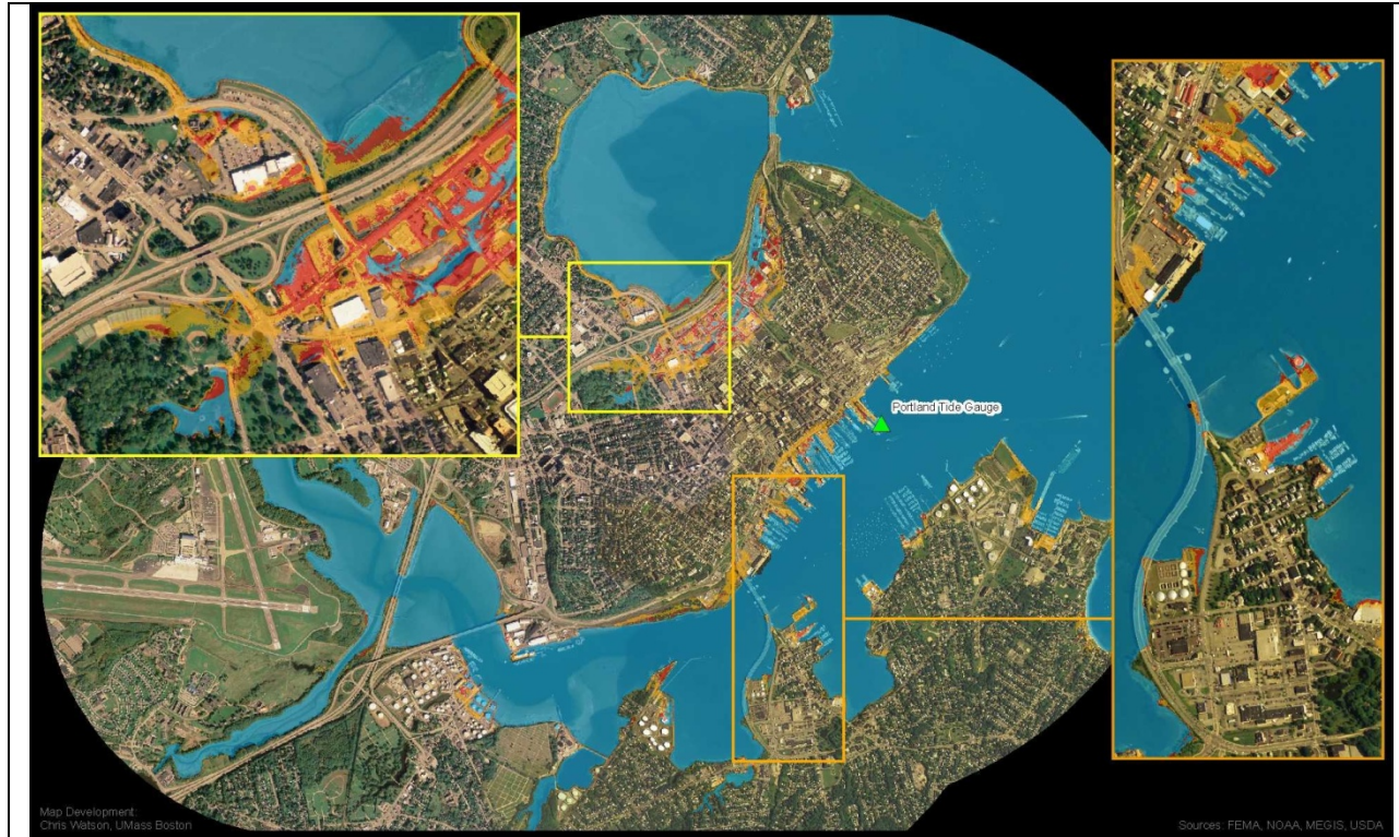
Figure 24. Shading indicates estimated flood areas near Portland Harbor during a 100-year storm in the year 2050 under a lower coastal flooding scenario. This map was developed using a five-foot by five-foot raster-based digital elevation model (DEM) overlaid on recent aerial orthophotography. The future elevation of the 100-year flood is based on the current elevation of the 100-year flood added to projected SLR. The lower coastal flooding scenario includes regional SLR due to land subsidence, and the low end of the range of eustatic (global) SLR projected by Rahmstorf xxxiv .
