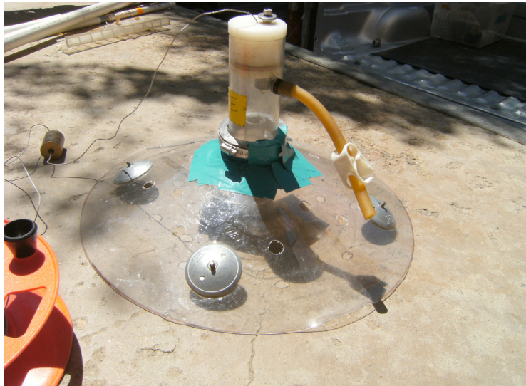
App. I, Fig. 2- Sediment “skimmer” used to collect benthic samples at Silver Lake, Hollis NH, on September 20, 2007
