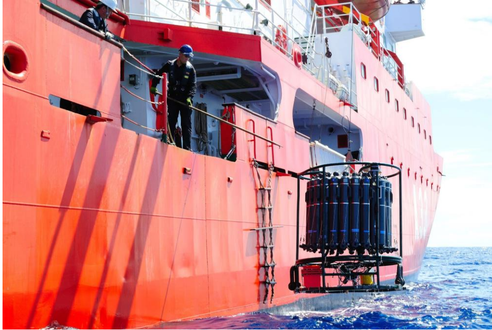
Figure 1.6. CTD rosette fitted with sampling bottles and sound speed profiler. Recovery after deep ocean dip. R/V Hesperides. (photo by the author)
