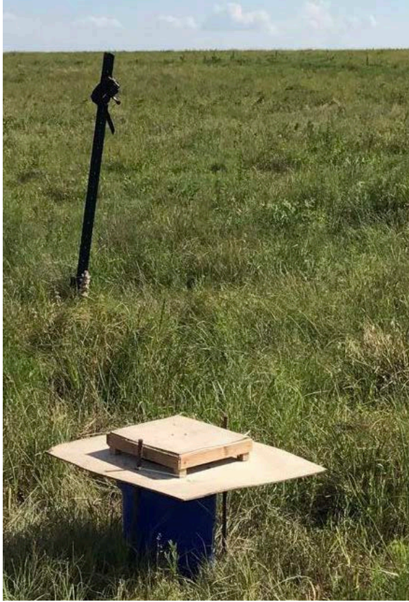
Fig. 1.2. Pictured is a typical sampling site which includes one above-ground pitfall trap (foreground) and one Arbimon portable recorder (Sieve Analytics, San Juan, PR) mounted to a temporary metal fence post situated 5-m away (background). Each recorder was placed askew so that the microphone would not interfere with the post from behind which may have been disturbed by wind or with the post itself by creating a notch in the frequency spectrum. All materials were removed at the completion of each trapping period.
