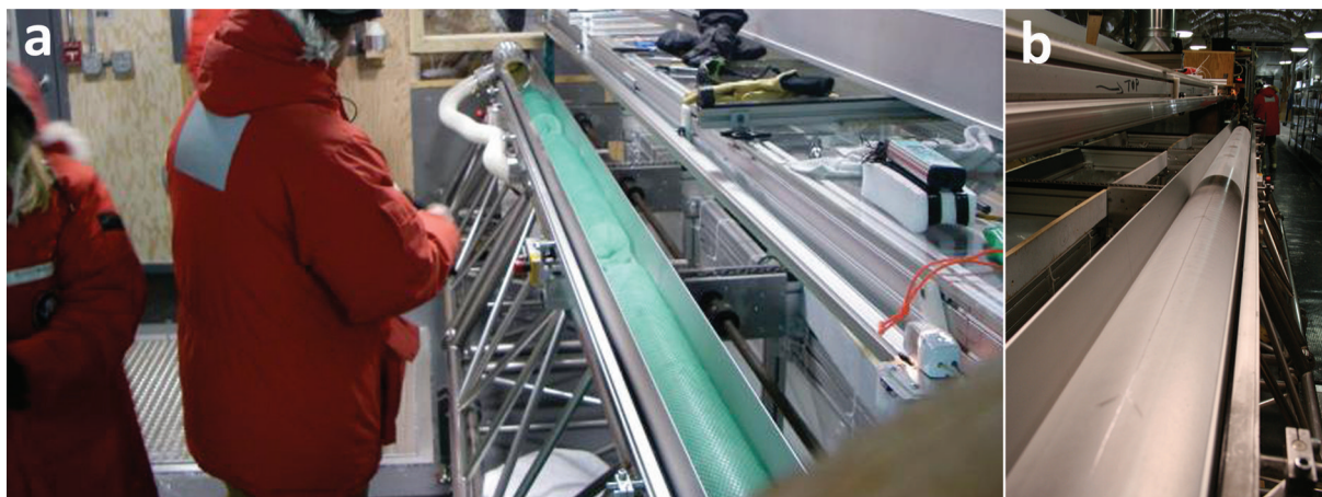
Fig. 11. View of the ‘Receiving and logging’ station at WAIS Divide with (a) 2.5 m of brittle ice contained in the green elastic netting and (b) a 3.2 m long continuous run of ductile ice showing one of the many prominent tephra layers observed in the WAIS Divide ice core.
