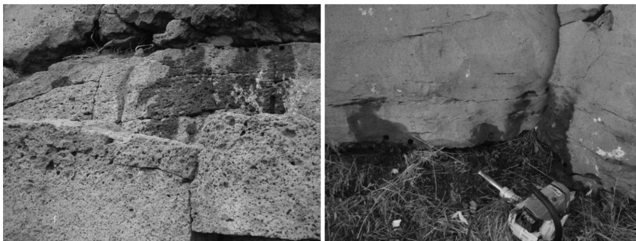
Figure 3. Coring locations at the top ( left ) and bottom ( right ) of a typical basaltic lava flow. Cores are 2.5 cm (1 inch) in diameter. Note that the upper vesicular zone contains many large, coalesced vesicles, while the lower vesicular zone has smaller vesicles and no coalescence. A massive zone separates the two vesicular zones. The darkened areas are wet from the drill-cooling water. A color version of this figure is available online.
