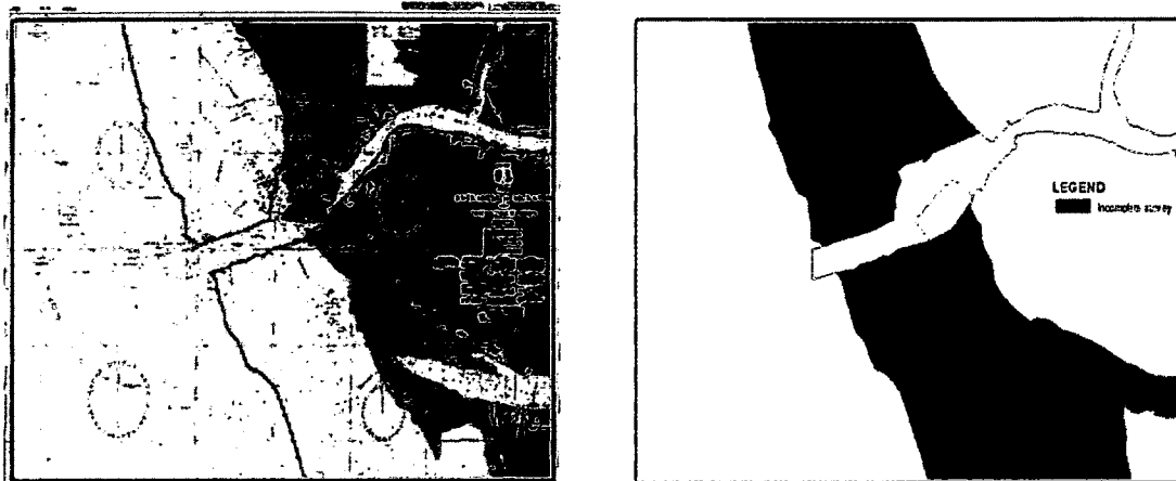
Figure 2.11 Incomplete survey: (left) BA Chart 3321 showing general area of incomplete survey and (right) polygons showing areas of incomplete survey.
