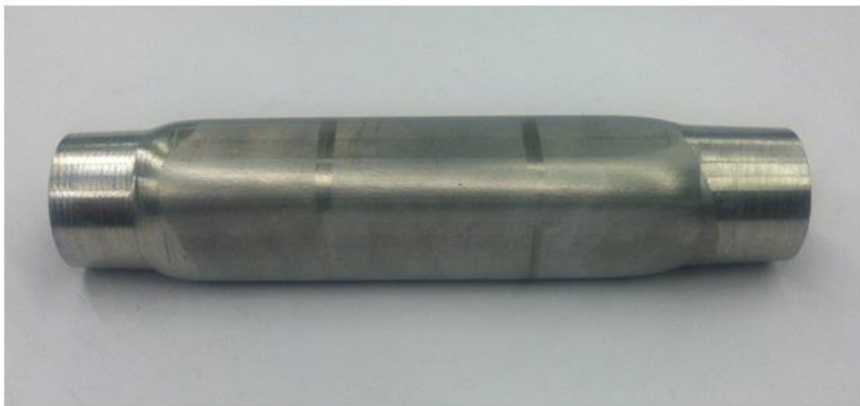
Figure 1.14: Hydroformed Al-6061-T4 tubes from the table-top hydroforming machine at UNH.
