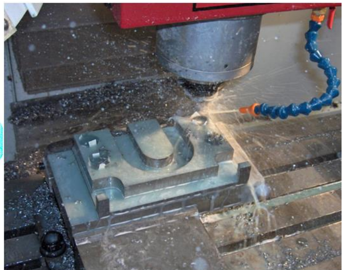
Figure 2.15: An example of the CNC machining being performed at the UNH CEPS machine shop on the Fryer MC-10.
