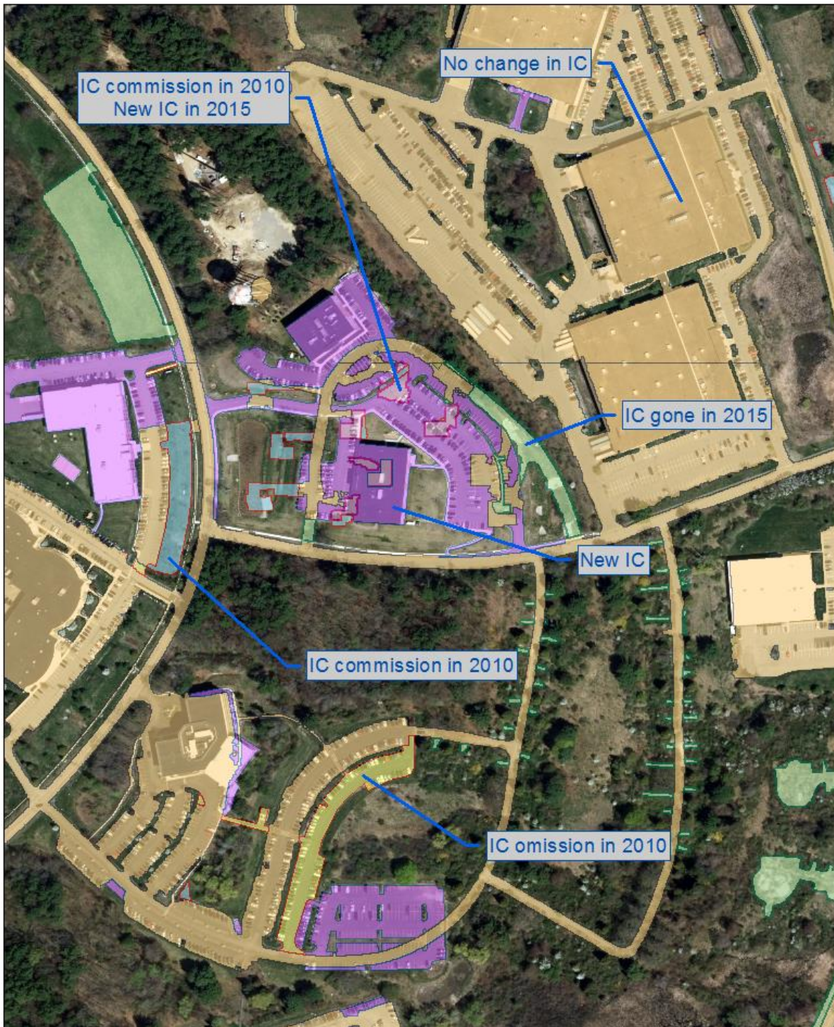
Figure 3. Examples of impervious cover change between 2010 and 2015.
