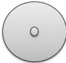
Figure 2.16: Single mode fiber
