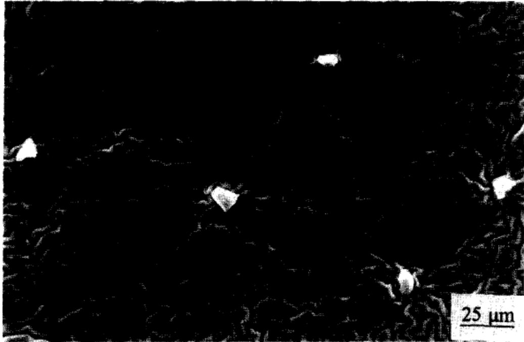
Fig. 2.29. Scanning electron micrograph showing the surface of the MMC before exposure to saline solution: the surface was originally in contact with lacquer during preparation of the MMC [13].
