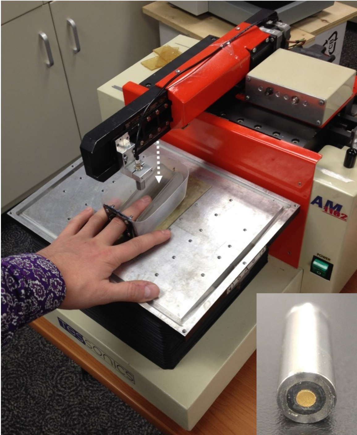
Figure 5.2: Setup used to obtain the thickness of fingernail using ultrasound in V(z) mode. The dashed arrow indicates the direction of motion on the transducer. The bottom right image shows the transducer where the gold circular area is the aperture surface.
