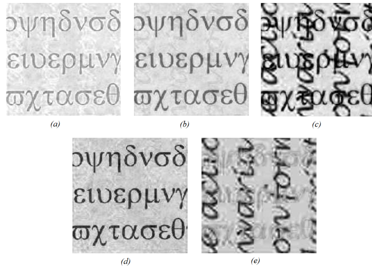
FIGURE 1.5: separation of overwriting and underwriting from an RGB real-fake palimpsest. (a) the red channel; (b) the green channel; (c) the blue channel; (d) first separated text; (e) second separated text [36]
