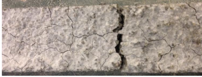
Figure 2.10. Deteriorated CG specimen immersed in NaOH solution for 14 days
