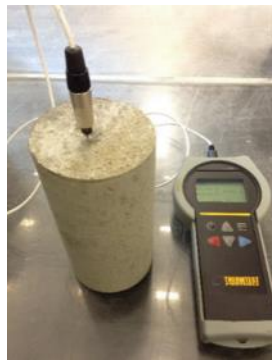
Figure 3.5. Testing procedure for thermal conductivity
