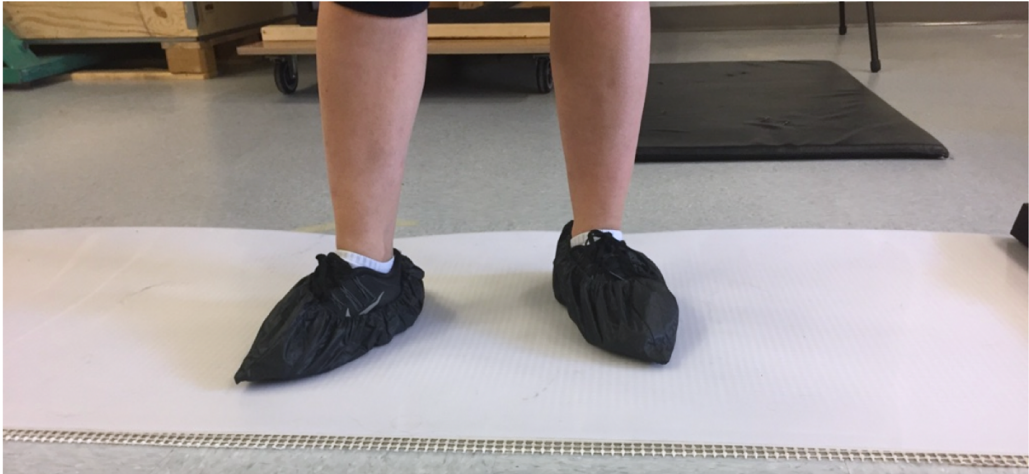
Figure 9: “Speed Booties” to be worn during sliding in order to reduce friction.
