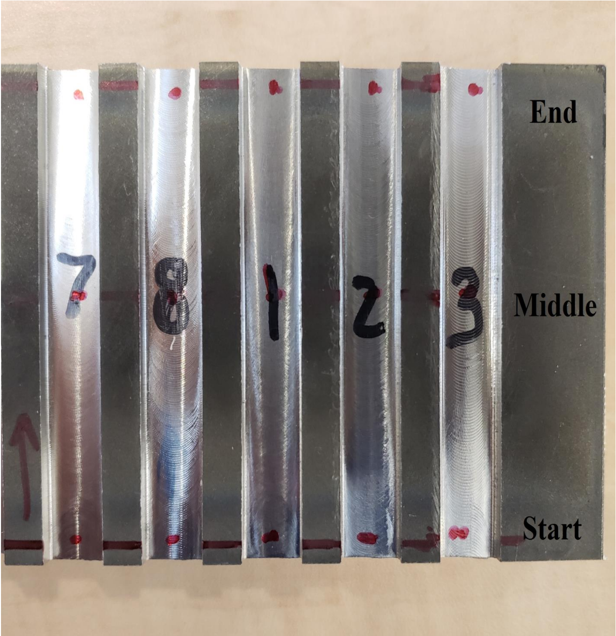
Figure 4.1 Marked bar of Inconel 718 for measuring of surface roughness.
