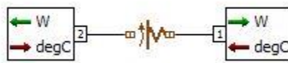
Figure C- 4: AMESim sub-model THGCV2 models the convective heat transfer between a fluid and a material [27].
