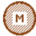
Figure B- 2: AMESim icon for sub-model THSD00 which provides thermal properties for solid materials, the user can use the pre-defined material, the user-defined material with constant thermal properties or the user-defined material with thermal properties vary with temperature [27].
